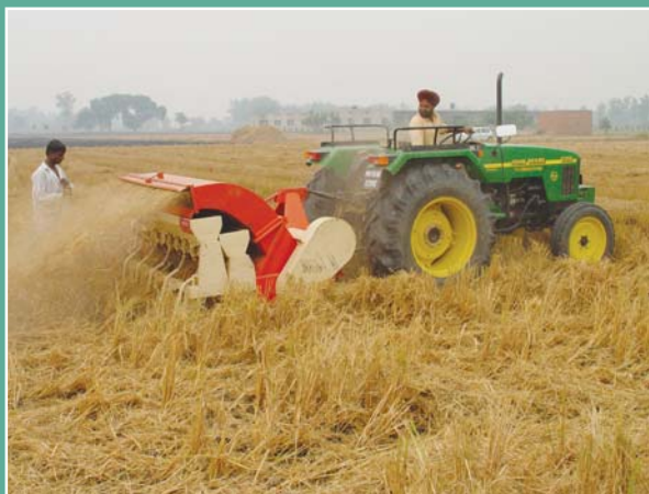
Figure 3 Direct drilling wheat into rice residues with the Combo+ Happy Seeder
