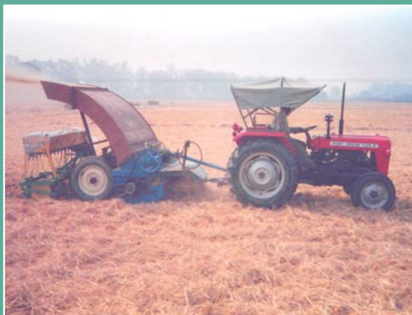
Figure 1 The original Happy Seeder concept in Punjab, India – a 35 hp tractor successfully sowing into 6.5 t/ha spread rice straw
