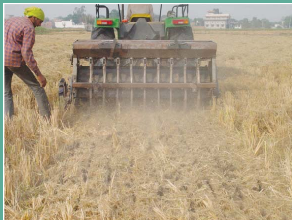
Figure 4 The Turbo Happy Seeder with seed rows left relatively exposed – hopefully a big advantage for establishment, especially for sowing into rice stubbles
