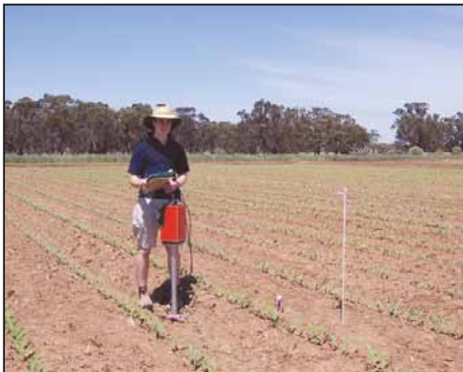
Figure 2: Crop establishment and Chris O'Neill taking neutron counts for determining soil water content
