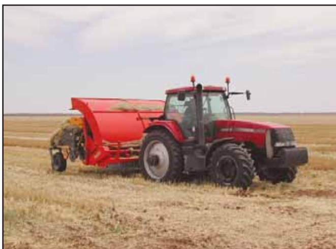
Figure 5: A prototype seeder that may eventually help farmers deal with the issue of stubble retention in intensive systems
