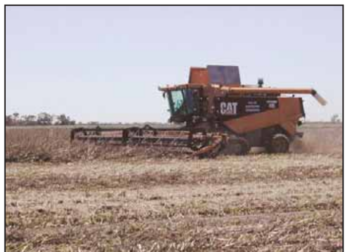
Figure 2: Harvesters can now be configured for controlled traffic systems such as this one harvesting faba beans
