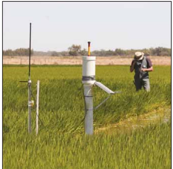
Figure 3: Automated temperature and water depth sensor (foreground) in cold tolerance plots at Old Coree and Peter Snell in the background tagging flowering rice panicles.
