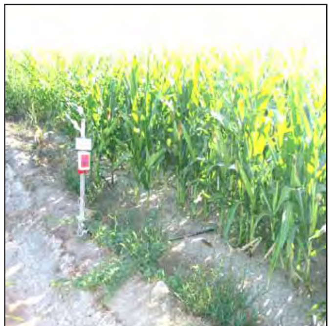
Figure 2: A GBug data logger and wireless retriever (in a maize crop).
