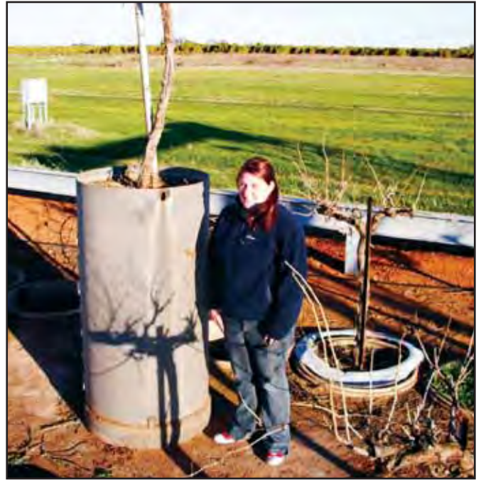
Figure 4: CRC for Irrigation Futures PhD Student Belinda Kerridge standing next to one of the twelve 1500 kg weighing lysimeters currently being constructed at CSIRO Griffith to calibrate grape vine sap flow sensors
