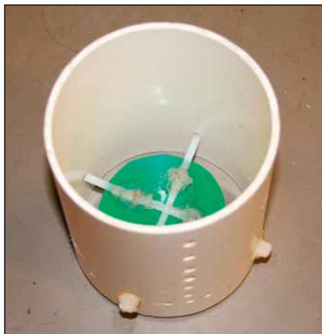
Figure 1: PVC soil corer used for collecting sediment samples. Holes on the side let excess water drain away, whilst the green plastic disc ensures samples are taken to a uniform depth.
