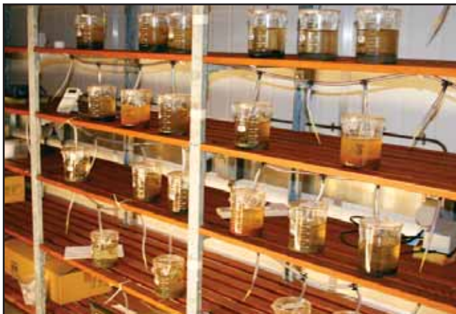
Figure 2: Replicated midge bioassays take place under controlled conditions using field-collected sediment samples.
