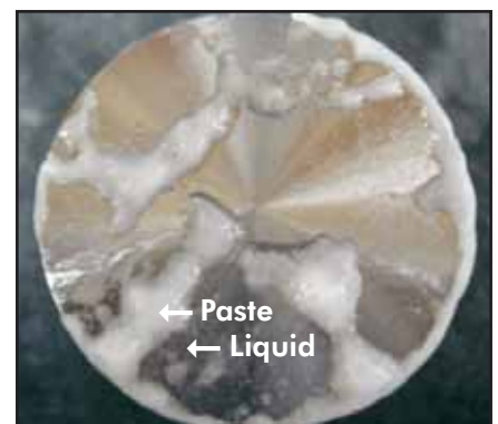
Figure 4: Phase separation of the low-viscosity sample into a soluble liquid and an insoluble paste.
