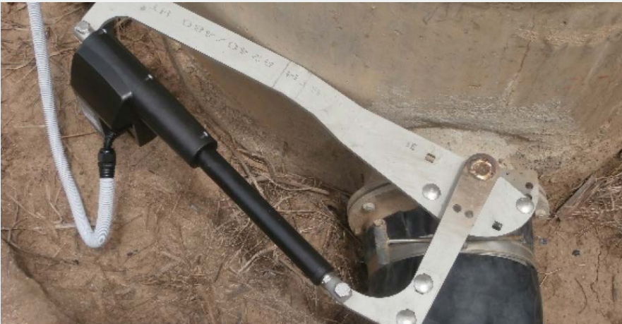
Figure 3. Linear actuators are used to open and close the various types of valves. Brackets are designed to retrofit existing infrastructure.
