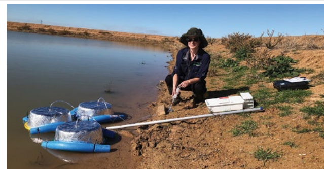
Dr Jackie Webb taking a gas sample from a floating chamber that measures greenhouse gas flux. Photo: Rakesh Awale
