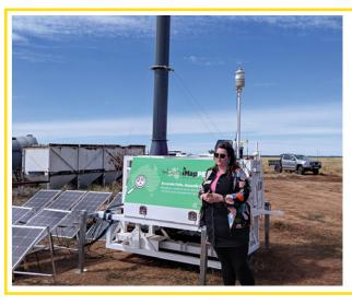
Shakira Johnson, AUSVEG, introduced the iMapPests project, which uses tall mobile surveillance units termed 'sentinels' that are topped with airborne trapping equipment and technology.
