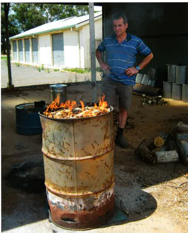
Figure 2. The combustion chamber is packed with pine chips that act as the fuel to generate high levels of heat around the inner chamber that contains the biomass that will become biochar.
