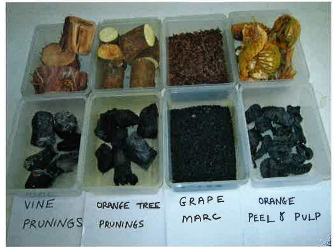
Figure 5. Biomass feedstock (upper row) and biochar products (lower row) produced in the small scale biochar maker.
