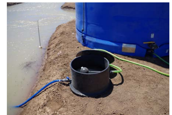
Example of a "header tank" for water running Urea 26.
